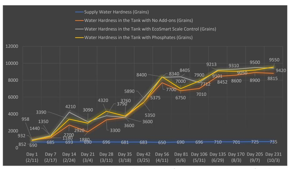
In the Figure above, we can see the supplied water hardness ranged from 650 to 735 over the course of 231 days.
